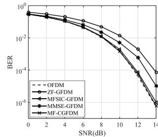
Fig. 2. BER of OFDM, GFDM receivers and MF-CGFDM in AWGN channel.
