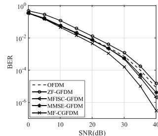
Fig. 3. BER of OFDM, GFDM receivers and MF-CGFDM in frequency selective channel.
