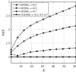
Fig. 1. NEF of GFDM and CGFDM for different values of  $K$  and roll-off-factor  $\alpha$ .
